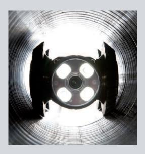
operate fully submersed and are water resistant to depths of up to 100m. They are constructed from brass and stainless steel and are built with powerful 50 or 100W motors that can move through almost any pipeline system. The integrated sensitive inclinometer and the multi-frequency sonde allow you to map pipeline topography easily and efficiently.
